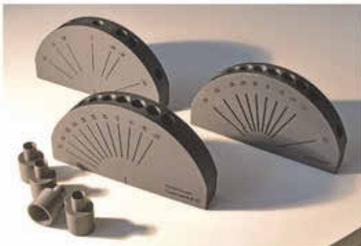
图6：带有灯适配器的GonioViewer 02* Figure 6: The GonioViewer 02 with adapter for a lamp.
